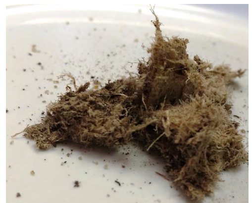
Figure 2 Friable test – example of hand crumbled low density fibre board found in soil originally in a rectangular form (FA).
