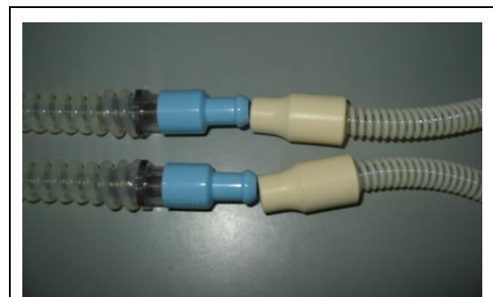
FIG 9 - Connectors between extension configuration tubing and ventilator circuit
